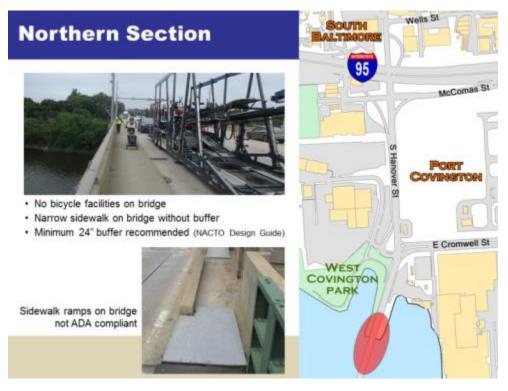
FIGURE 4-10: MULTIMODAL BARRIERS NORTH OF THE DRAWBRIDGE SPAN (3)
