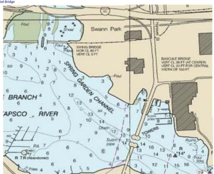
FIGURE 4-18: MIDDLE BRANCH WATER DEPTHS AND VERTICAL CLEARANCE
