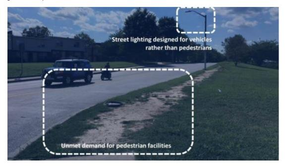
FIGURE 4-4: MISSING PEDESTRIAN NETWORK LINK AND VEHICULAR LIGHTING
